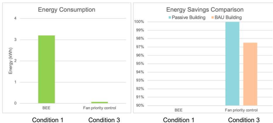
Figure 7: Energy Analysis Results, energy consumption (total during the study period in both buildings), savings for the fan-priority control compared to BAU for each building.
